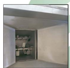
The drainage truck has been specifically designed to collect drainage from the ricotta produced from surfacing in the flocculator.
