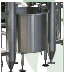
Autonomous system for ricotta production, which can process large quantities of whey or milk, significantly cutting down on labour and energy costs.
